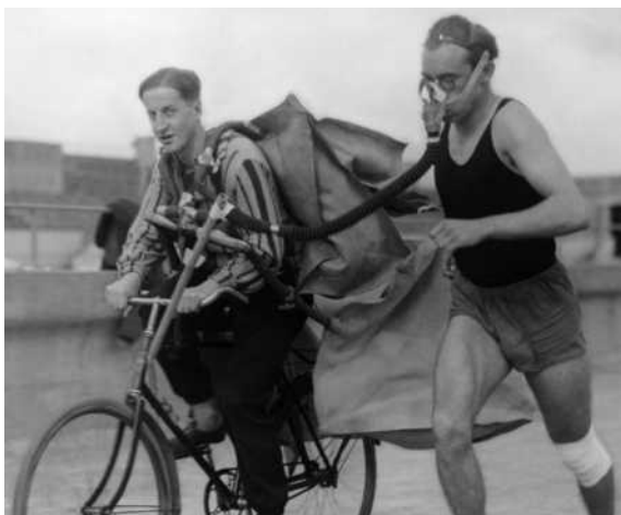
Figure 0.1 Comparison of old and new technology used to measure oxygen consumption and carbon dioxide production during exercise. (Right: COSMED.)
